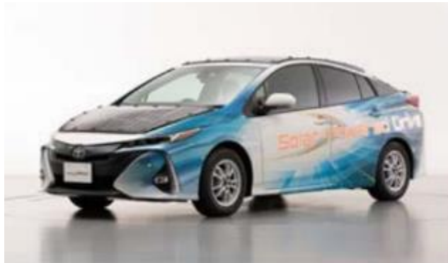
Test car – Multijunction PV on Prius
